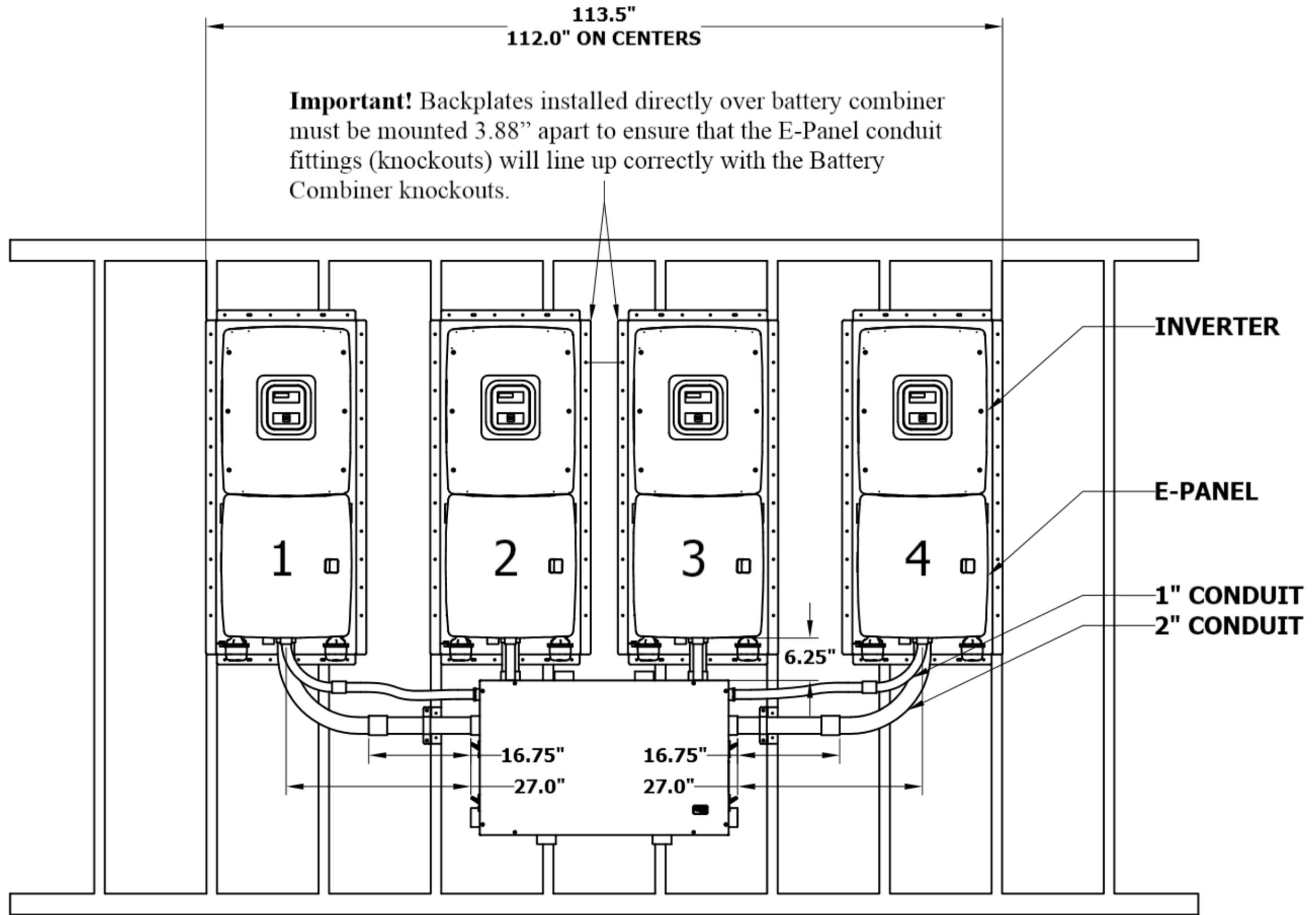
SMA QUAD WITH BATTERY COMBINER TYPICAL WALL MOUNTING
