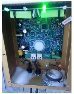
The PCB area of that same Birdhouse. The fine powdery snow had no trouble finding its way in through the unsealed edges. Some of the mounting holes were left unused providing more access to insects and the elements. The battery insulator tab was not removed either.
