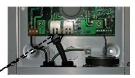
4. REMOVE the shunt from CON4 and place it in the shipping position until the entire installation procedure is completed to conserve battery power.
