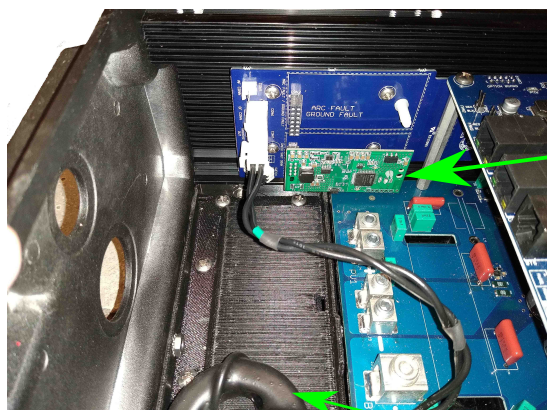
Barcelona charge controller with option board
