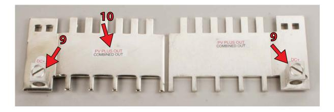
Step 9. Screw on the terminal blocks #9-075-1 on each busbar #3-174-1 using #6-059-1 screws and #6-017-1 lock washers.
