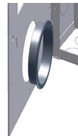
Figure 11, Installing 3.5" Grommet in the Door
