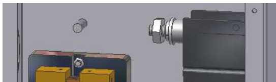
5/16" stud for battery negative tie point
