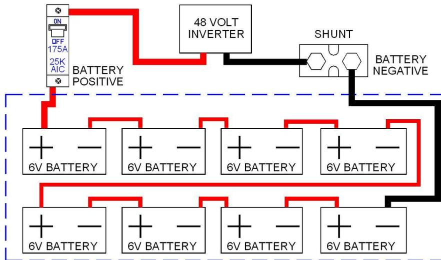
This configuration uses 6 volt sealed batteries that result in only one string. This is a 48 volt battery bank. You could add 3 more cabinets and have only 4 paralleled strings.
