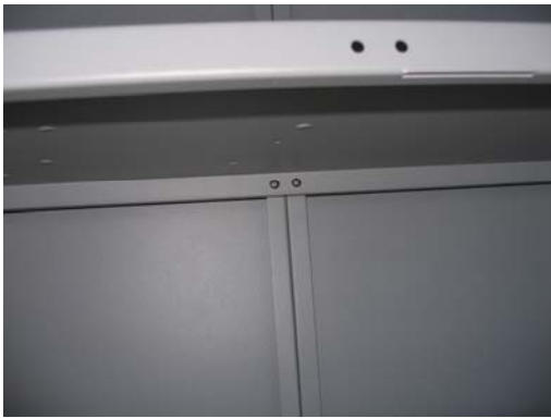
Two screws attach under each shelf to the backs from Step 3
