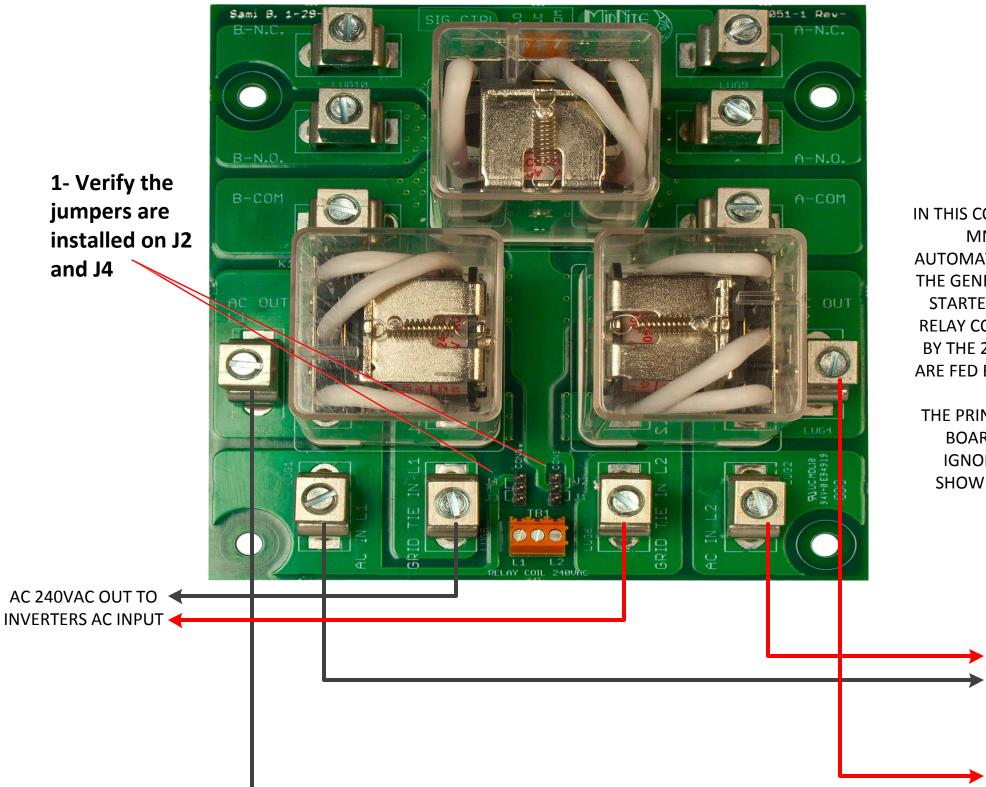
IN THIS CONFIGURATION THE MNTRB80 WILL AUTOMATICALLY SWITCH TO THE GENERATOR WHEN IT IS STARTED. BASICALLY THE **RELAY COILS ARE POWERED** BY THE 2 TERMINALS THAT ARE FED BY THE GENERATOR
