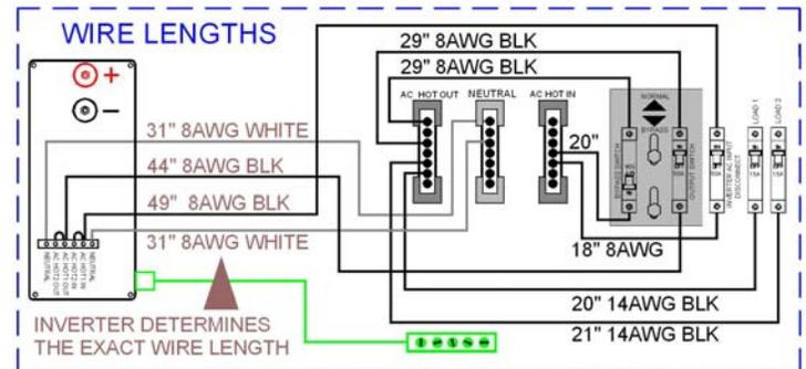
The diagram above shows wires that need to be cut, stripped and installed. Length, gauge and color is noted. Strip 3/8" for the end inserted into the din rail mount breakers. Strip 1/2" for the end inserted into the bus bars. The AC wire lengths going to the inverter are only a guideline. The length indicated will suffice for a Magnum Energy or OutBack inverter. Note that two white neutral wires are indicated to the inverter AC terminal strip. Magnum Energy 120VAC
