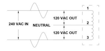
In this example the AutoFormer is being fed 240 Vac and is creating two opposite (180° degrees out of phase) 120 Vac taps
