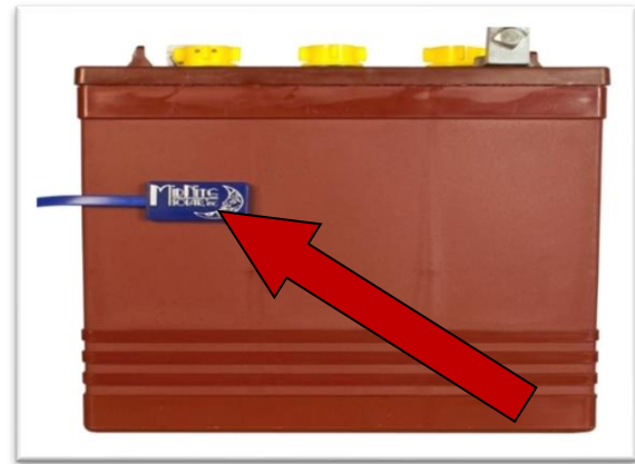
Figure 16 – Battery Temperature Sensor Mounting
