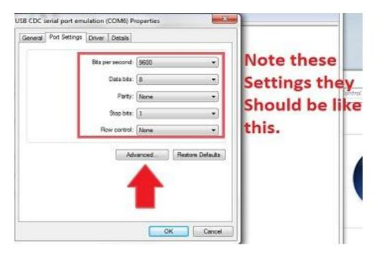
Step 27. Select the Com port and switch it to 8. Then Click Ok on this window and the one below it. And simply close out of all the Device Manager related stuff.
