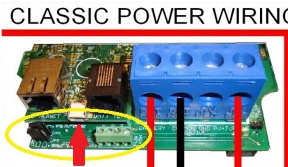
Step 13. With the power on to the Classic, plug the other end of the USB cable into the PC you are using to install firmware. The “Found new Hardware” window will open, Left Click on the Choice shown.
